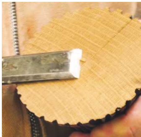
▲ Pic.20 Cut as much of the spigot away between centres as you can. Take the piece off the lathe and remove the last bit of timber with a sharp chisel
